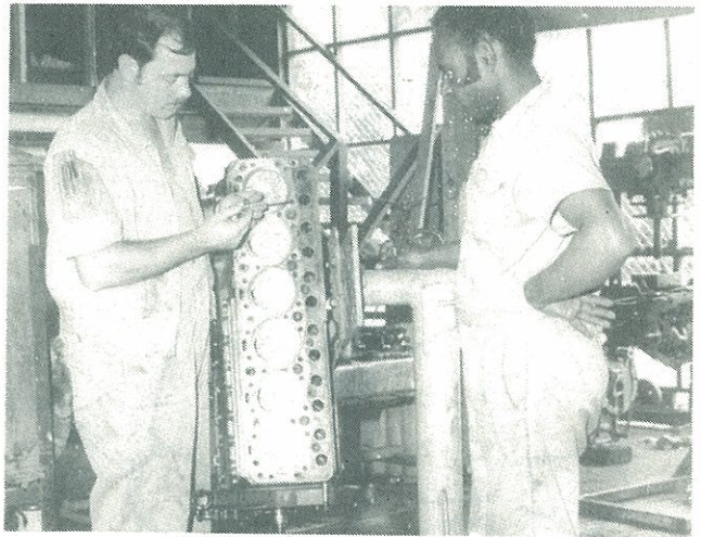
Cpl Barry Burt instructing senior casual mechanic, Mr Poya Kapie, on the use of an inside micrometer.
