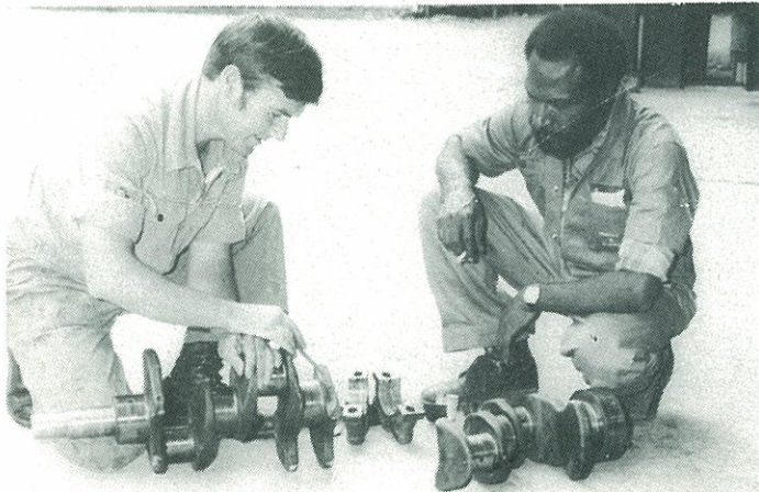
The author, WO1 Barry Woodberry and Plant Inspector, Karefa Komonome, inspect the broken crankshaft of a Komatsu D55S Tracked Loader.
