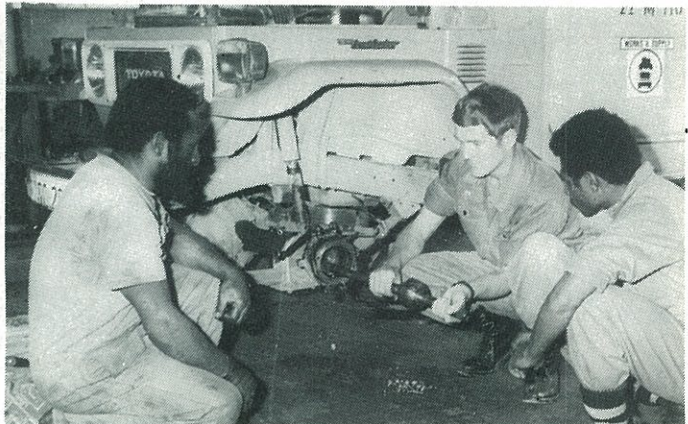
Our Training Supervisor, Sgt John Heafield, explains the operation of a Birfield Universal Joint to casual mechanic Mr Yamba Naripu (left) and Apprentice Orehere Kerere. The UJ is from a Toyota Landcruiser.
