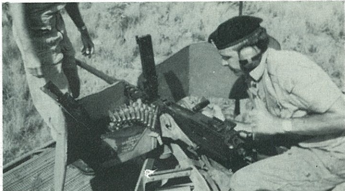
Lcpl Mason effecting repairs to a .50 calibre MG.
