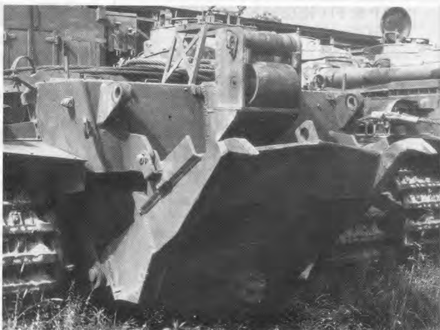
The rear anchor spade and fairlead assembly of the ARV Mark 1. The relatively light construction of the spade compared to that of the Mark 2 can be seen
