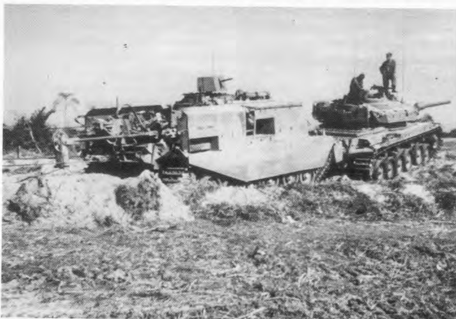
A Centurion ARV Mark 2 in South Vietnam during 1968. The anchor spade is embedded in the ground and the winch rope has been reeved into a 3 to 1 layout. A Centurion MBT has been hooked onto the front of the ARV to provide an additional anchor. The ARV has the rear deck protection plates fitted and a shield on the commander's machine gun
