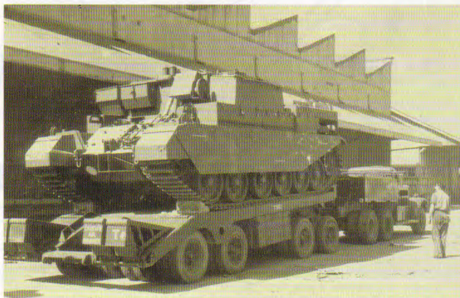
One of the first Centurion ARV Mark 2 to arrive in Australia during 1956. The vehicle is being carried on a Dyson 50 ton Tank Transporter trailer towed by an M20 Diamond T Prime Mover
