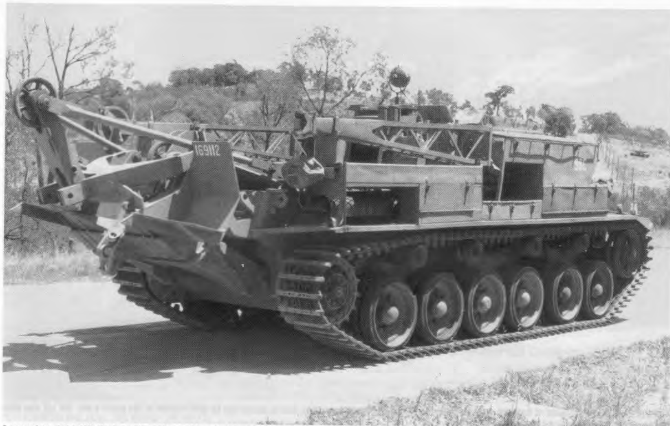
A rear view of the ARV Mark 2 with anchor spade raised in the travelling position. The rear jib can be seen as can the two sections of the lattice jib carried on top of the stowage boxes
