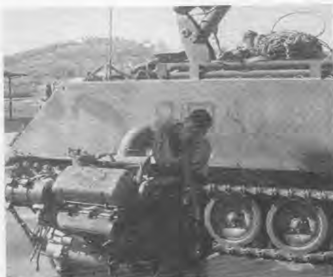
CFN Downey replacing a transmission on one of the buckets cars
