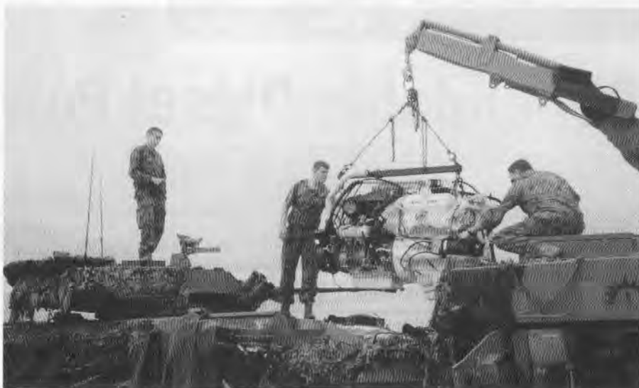
Left to right (on pack): CPL 'Phil' Wadley, CFN Glenn 'Old Man' Dunn - LAV Engine change
