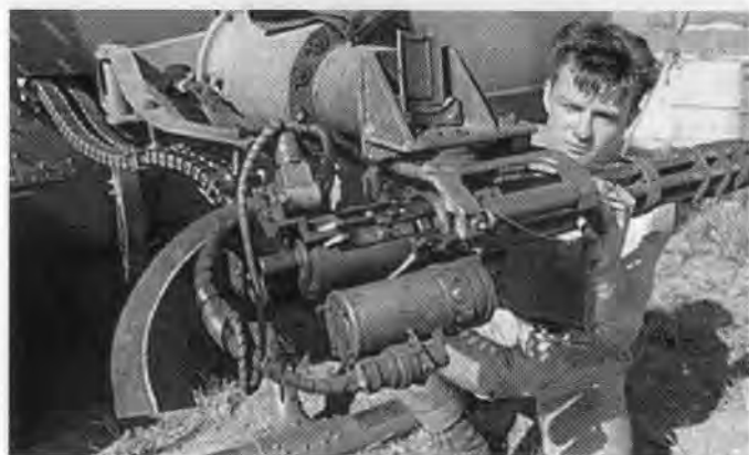
CFN 'Macca' McClure performing some scheduled maintenance on a mini gun fitter to an Iroquois Gun Ship
