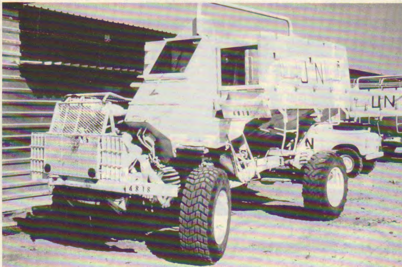
Due to the serious mine threat existing within Namibia twenty-four mine protected vehicles were purchased for UNTAG. The picture shows a Buffel vehicle which was a mine protected armoured plated drivers cabin and squad compartment mounted on a Unimog chassis. The Australian contingent became heavily involved with driver training and maintenance of this vehicle.
