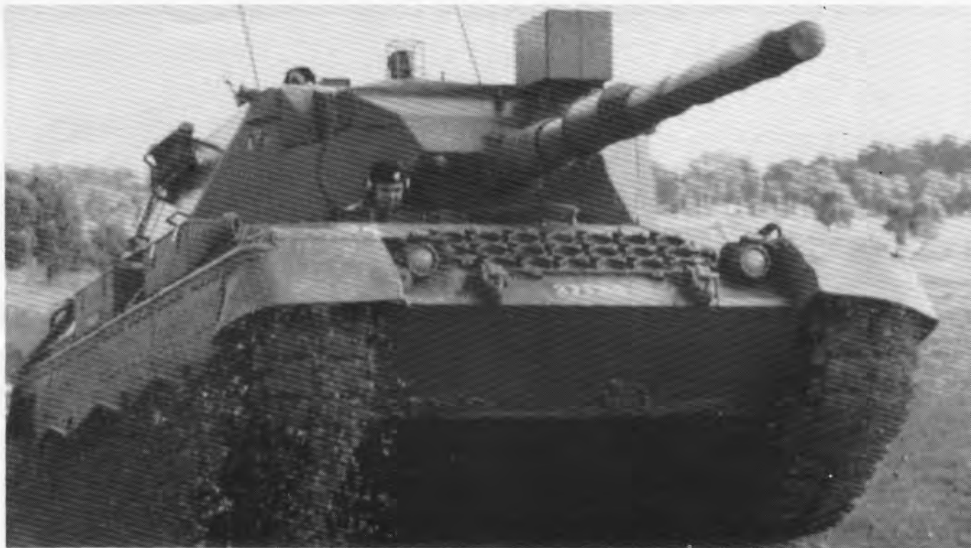
The Army's Leopard tanks exploit the high power-to-weight ratio of MTU's aluminium diesel engine.
