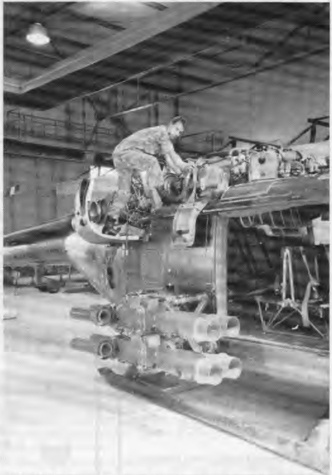
RAEME at work on Lynx transmission and Rolls Royce Gem engine.
