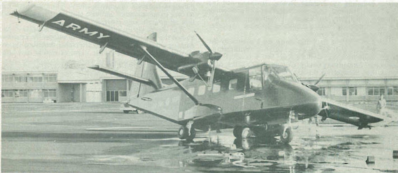
Nomad 306 with twisted undercarriage and extensive structural damage as a result of the winds.
