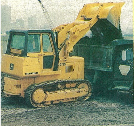
John Deere 755 hydrostatic drive loader.
