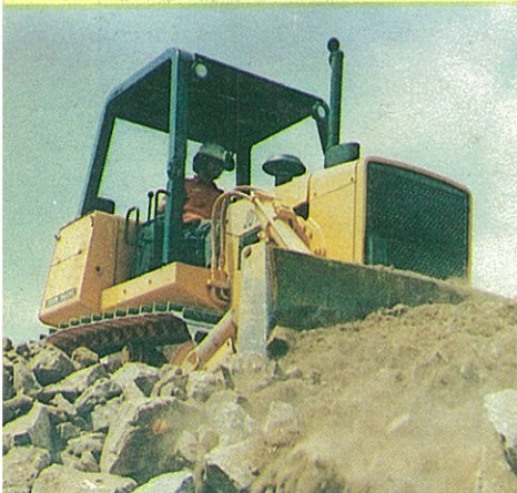
John Deere 850 hydrostatic drive dozer.
