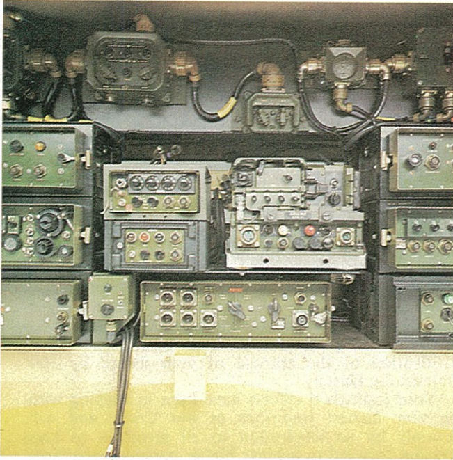
Two HF and two VHF radios in one vehicle? Racal has solved the EMC problems.
