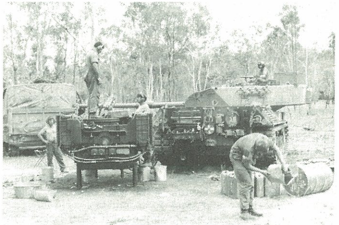
33A being run up after over 200 hrs work to recover power pack.
