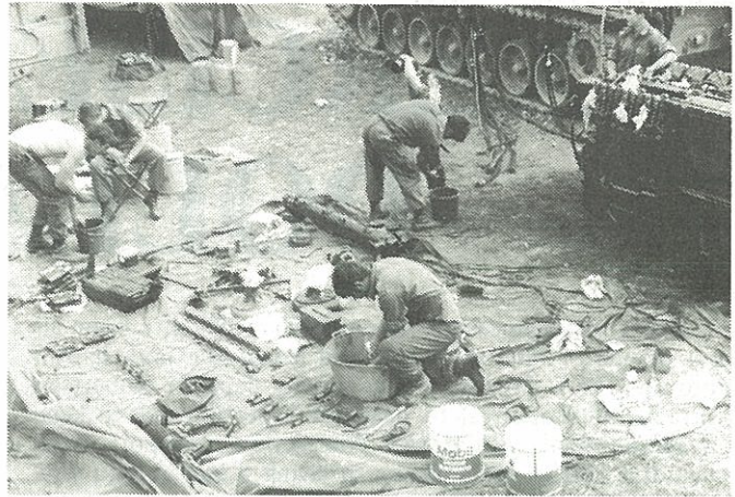
Busy Tech Support crew cleaning parts of 33A's power pack.
