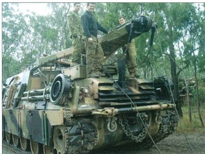
1 AR bogologists changing M88 winch rope in the rain. Recce Mech porn!
