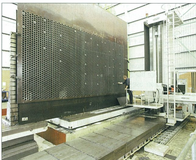
Baker & Provan's 12 metre CNC Floor Borer makes Baker & Provan one of the large and modern CNC machine shops in Australia. The Floor Borer has a machining envelope of 12 metres across, up to 4 metres high and can handle work pieces up to 100 tonne on its 12 metre bed. The image shown is a large heat exchanger end plate for a power station.
