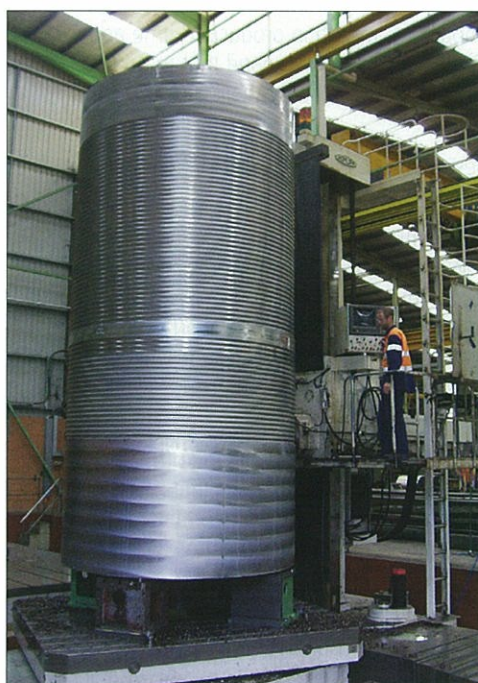
The 30 Tonne CNC turn table provides Baker & Provan a machine with 6 axis control. The machining height of this CNC controlled turn table is 4 metres high. The image shown is the machining of a heavy duty winch drum, which was fabricated and machined by Baker & Provan.
