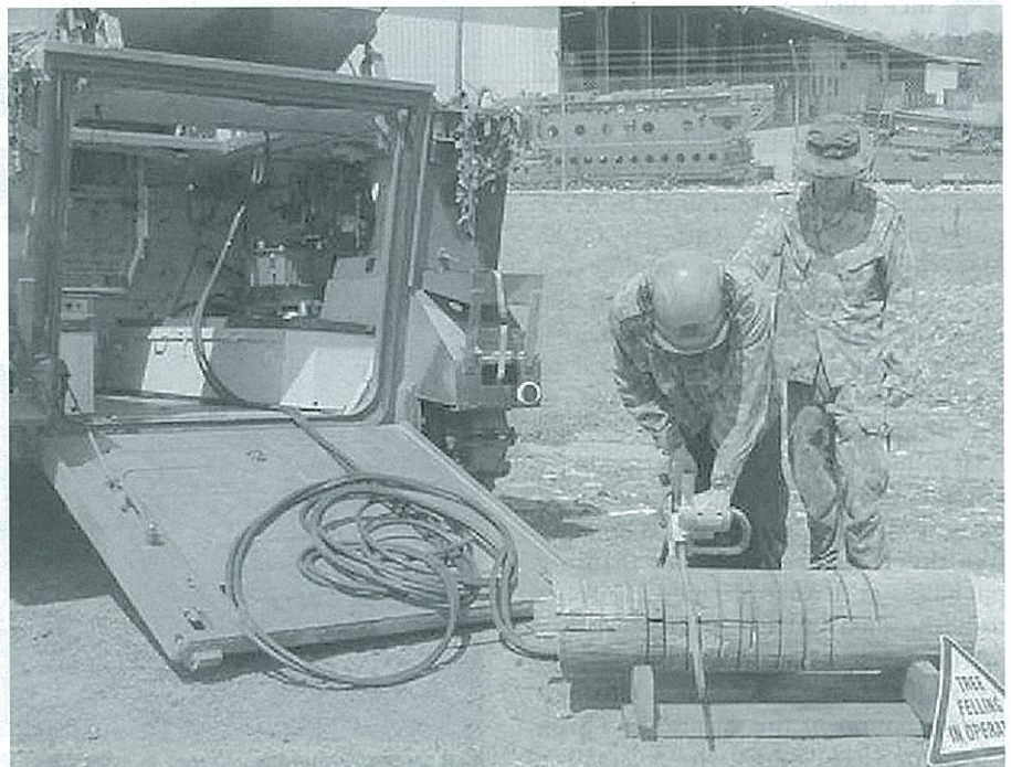
One of the many hydraulic attachments that can be powered by the M113
