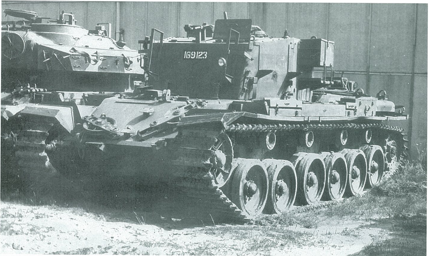
The ARV Mark 1 photographed at Bandiana after its withdrawal from service in late 1975. Snatch blocks can be seen stowed on the glacis plate. The tall slab-sided structure housed the winch and the Bedford engine
