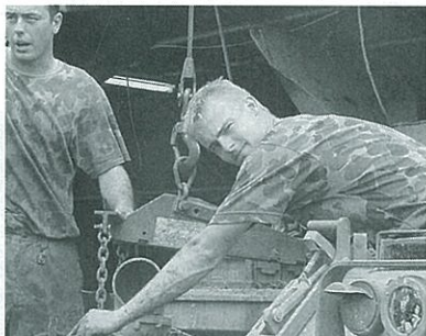
CFNs Vaughan and Zimpel conducting a powerpack lift
