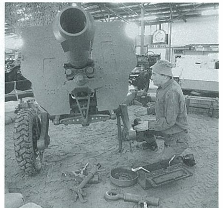
A section of the RAEME display featuring a gun repair task in the field in Vietnam
