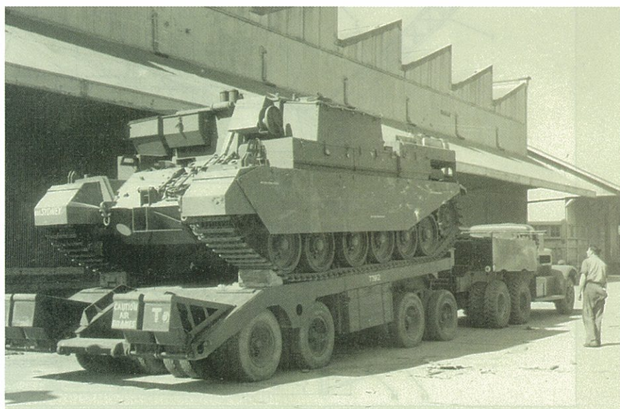
One of the first Centurion ARV Mark 2 to arrive in Australia during 1956. The vehicle is being carried on a Dyson 50 ton Tank Transporter trailer towed by an M20 Diamond T Prime Mover
