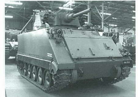
Fire Support Vehicle with Saladin Turret and 76mm Gun
