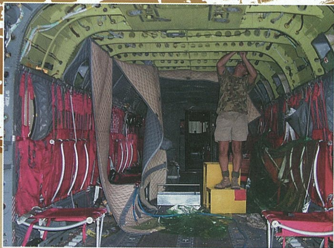
Tradesman conducting a repair to the fuselage skin
