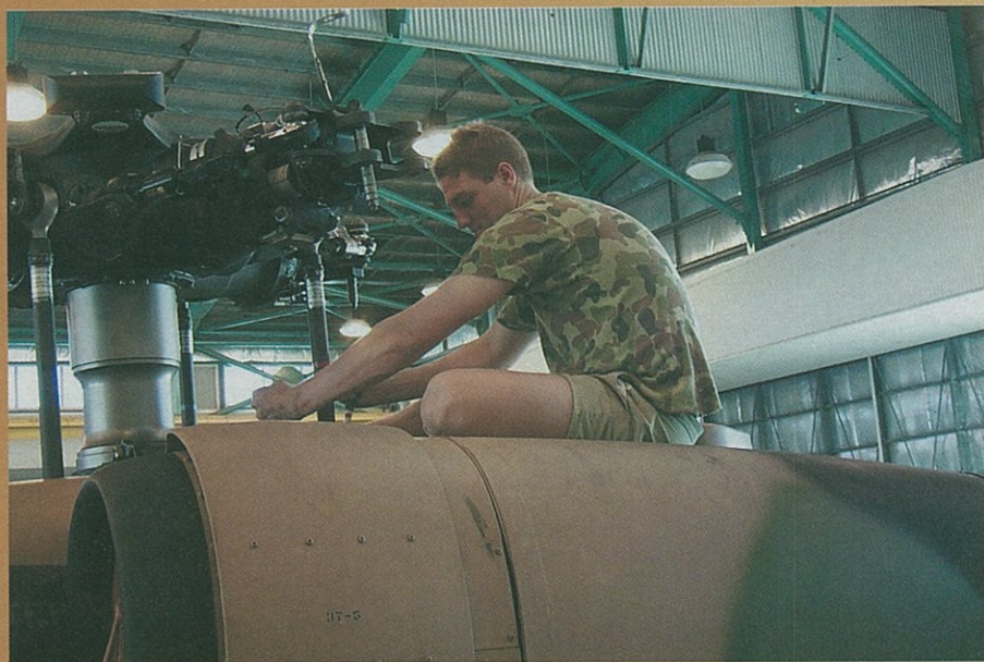
CFN Lonergan working on Blackhawk Rotor Head
