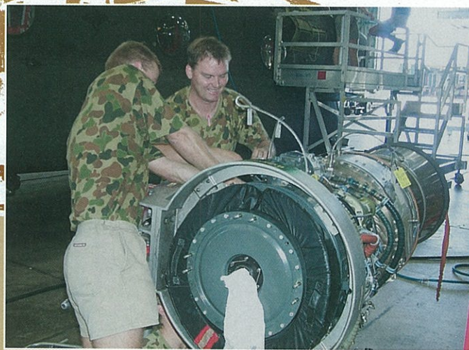
Tradesman conducting maintenance on a Chinook Engine (Lycoming T55-L-712)
