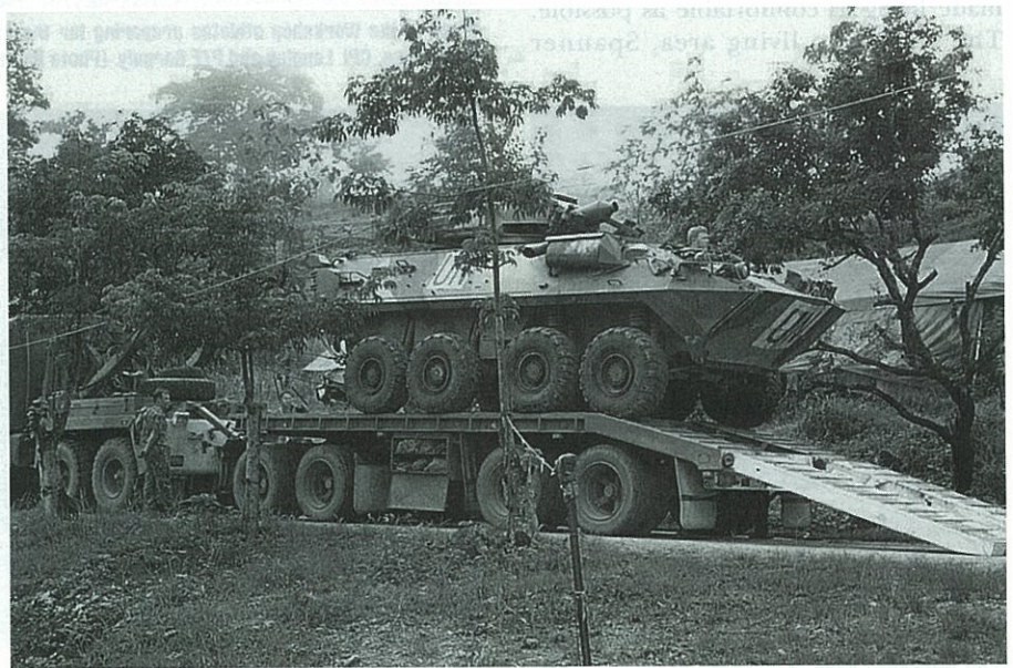
An ASLAV is winched onto the trailer of the HRV for return to Hera and then back to Australia. (Photo by CPL Peter Seabourne)
