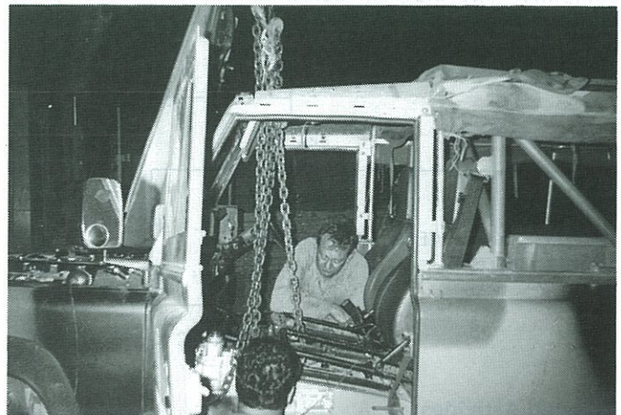
CPL B. Rae replacing a LR 100 GS gearbox at Oakleigh Barracks workshop.
