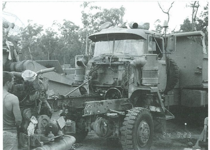
Replacing an engine and clutch on a Mack Dump at Scherger
