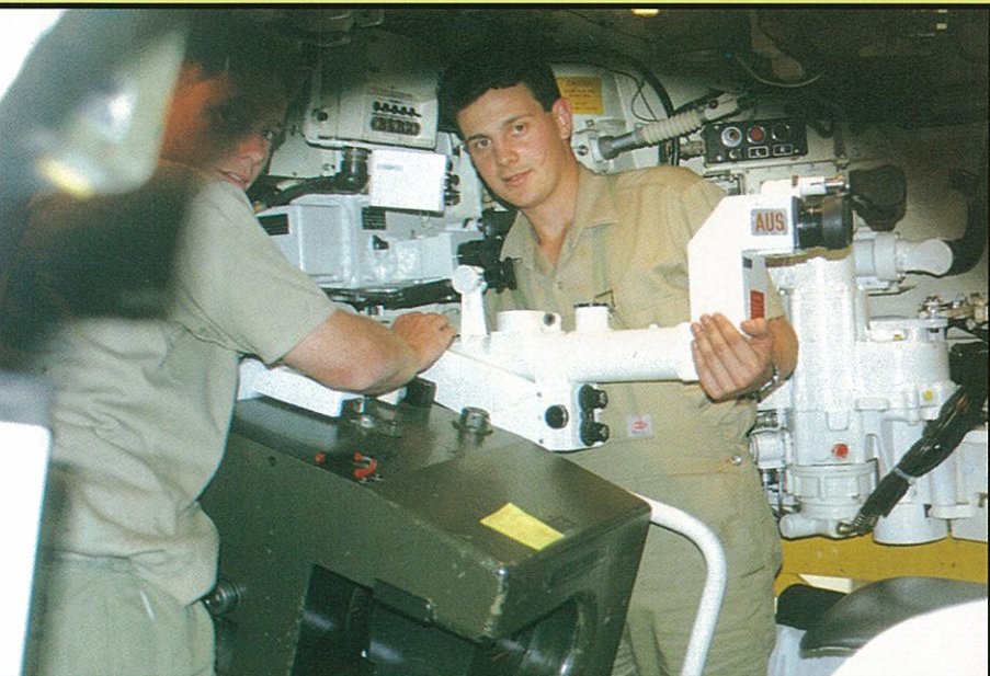
Centre L to R: CFN D. Hicks and CFN J. Claridge from the BLG fitting a Secondary Gunners Sight to a Leopard Turret as part of their On-Job-Training program.
