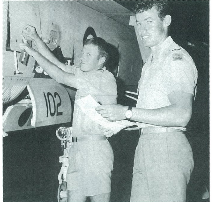
SGT G. Hall and CFN Paterson applying thermal strips to FA-18.
