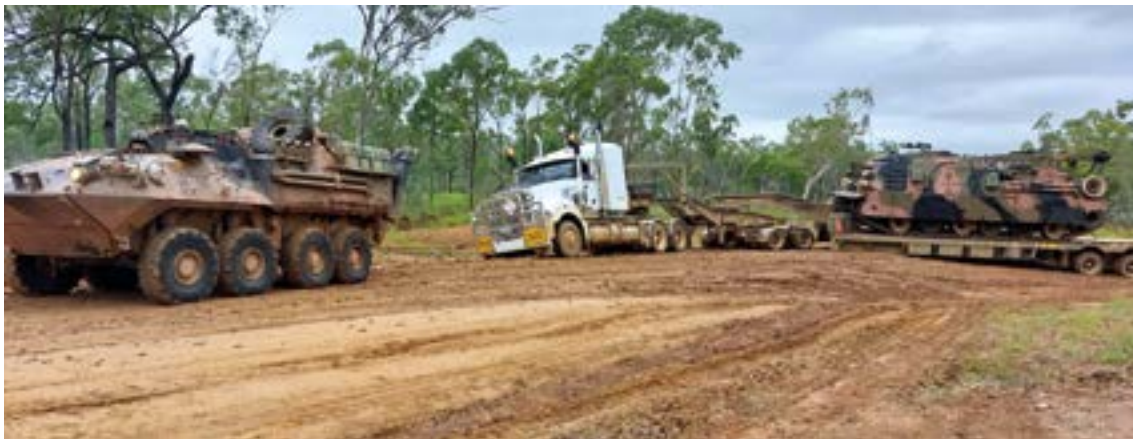
Recovery at work: B SQN ASLAV-R recovering a HTT that is recovering an M88A2
