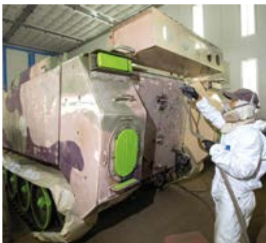
JLU(SQ) tradesmen painting & fitting Armour to the M113AS4
