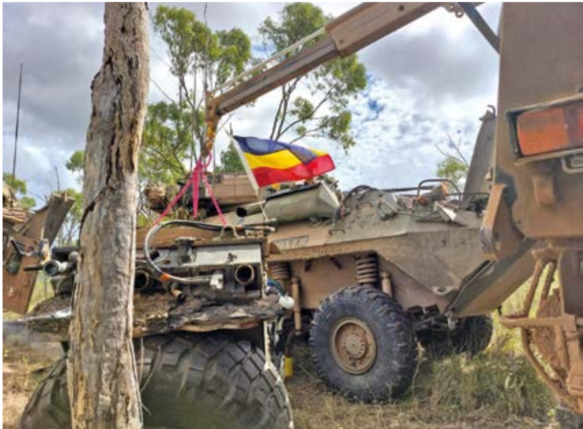
B SQN ASLAV Power Pack Removal – Ex SIDON
