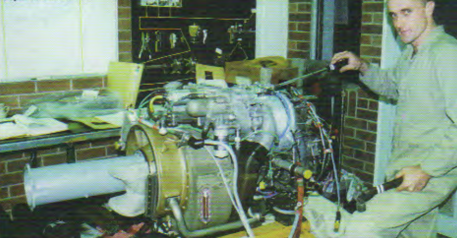
The engines are also dismantled, inspected, repaired and rebuilt
