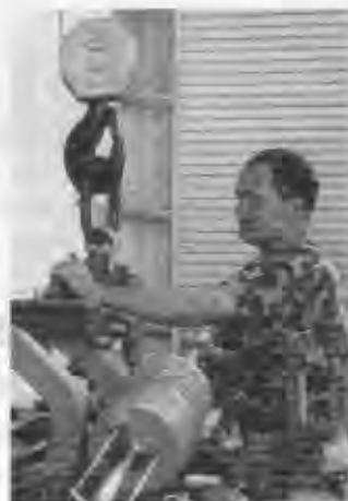
SGT J. Taylor replacing the ordnance of the 105mm Hamel gun
