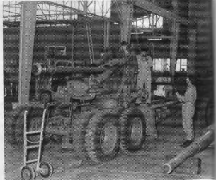
Changing barrel on M1 Gun Carriage CFN Coney, CFN Hoffman, Terry Nowland, John Dunn
