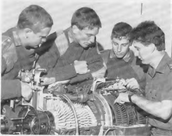
CPL McCrabb works through a demonstration on inspecting a turbo shaft engine.
